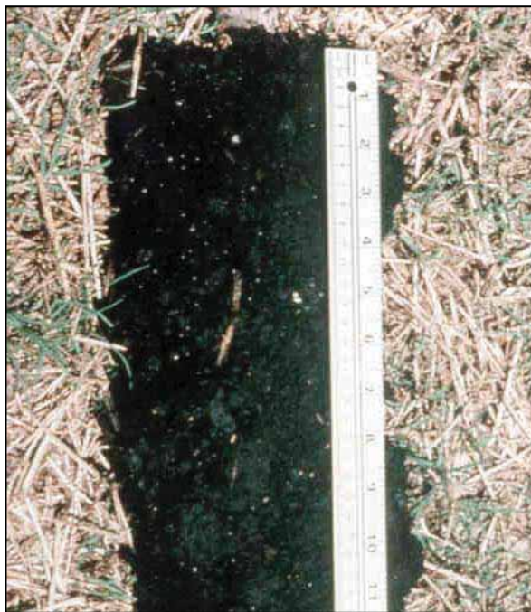
Figure 8. A black organic surface layer greater than 11 in. (28 cm) thick.
