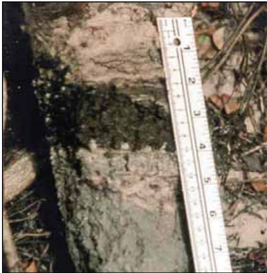
Figure 9. Stratified layers in loamy material.
