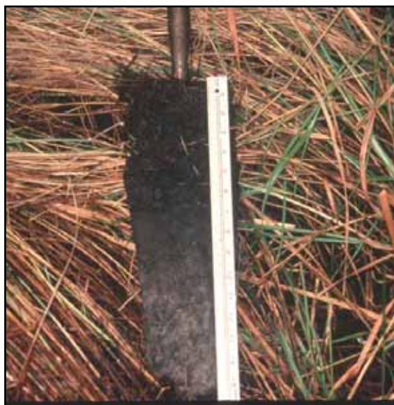
Figure 14. The mucky modified sandy layer is approximately 3 in. (7.5 cm) thick. Scale in inches on the right side of ruler.
