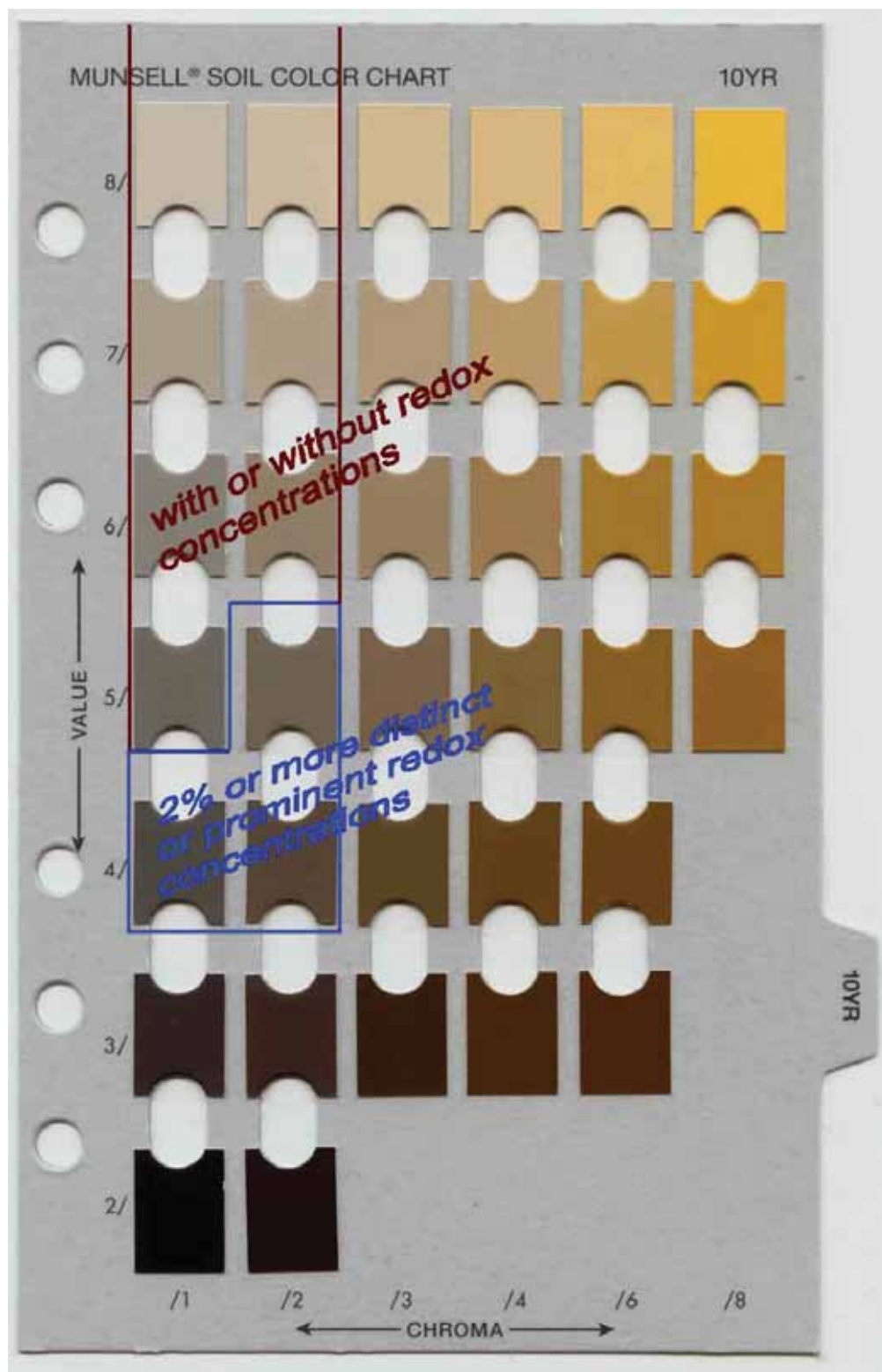
Figure A1. Illustration of values and chromas that require 2 percent or more distinct or prominent redox concentrations and those that do not, for hue 10YR, to meet the definition of a depleted matrix. Due to inaccurate color reproduction, do not use this page to determine soil colors in the field. Background image from the Munsell Soil Color Charts reprinted courtesy of Munsell Color Services Lab, a part of X-Rite, Inc.
