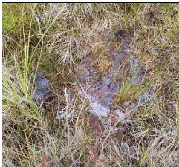
Figure 32. Iron sheen on the water surface may be deposited as an orange or yellow crust after dewatering.
