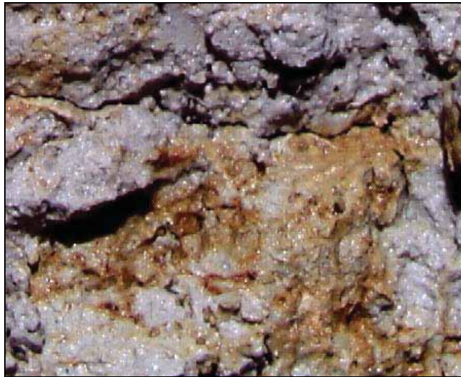
Figure 26. Water glistens on the surface of a saturated soil sample.
