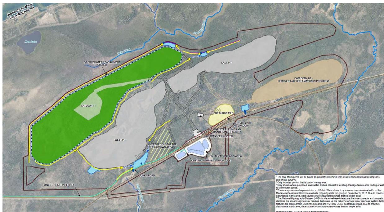
**Figure 7 Stormwater Ponds (in Blue) Around the Perimeter of the Mine Site**
