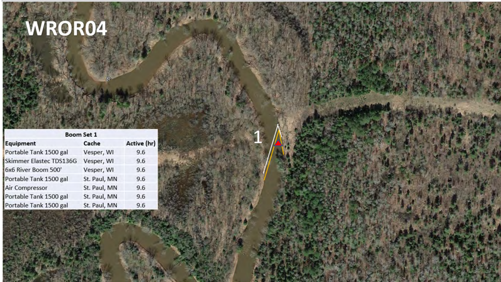
Figure 3-28. Response layout for MCP WROR04 on the White River. Red triangles are skimmer placement locations, orange lines represent containment boom, and white lines represent sorbent boom. The sorbent boom was not simulated in the model.
