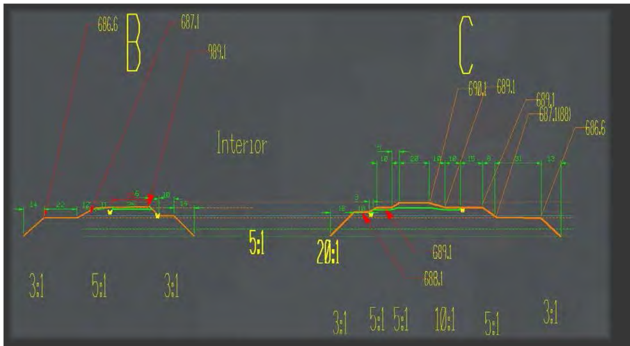
Figure 13 Split Island Cross Sections
