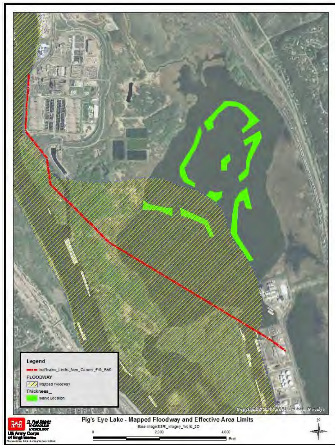
Figure 10 Mapped Floodway and Effective Flow Area Limits
