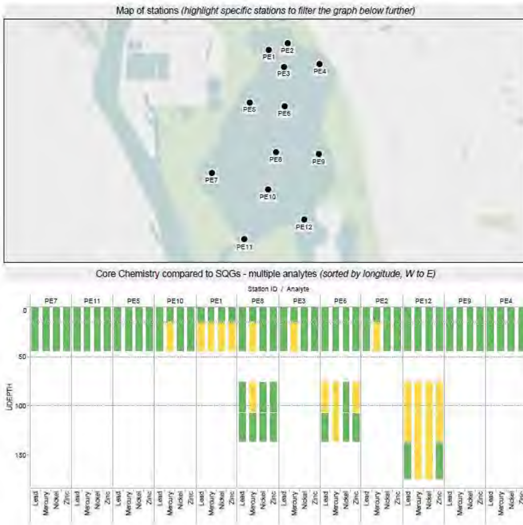
Figure 2. Spatial distribution of SGT I exceedances for mercury, lead, nickel and zinc. MPCA 2007-2008 survey (green = below SGT level I, yellow = between level I and level II SGT)
