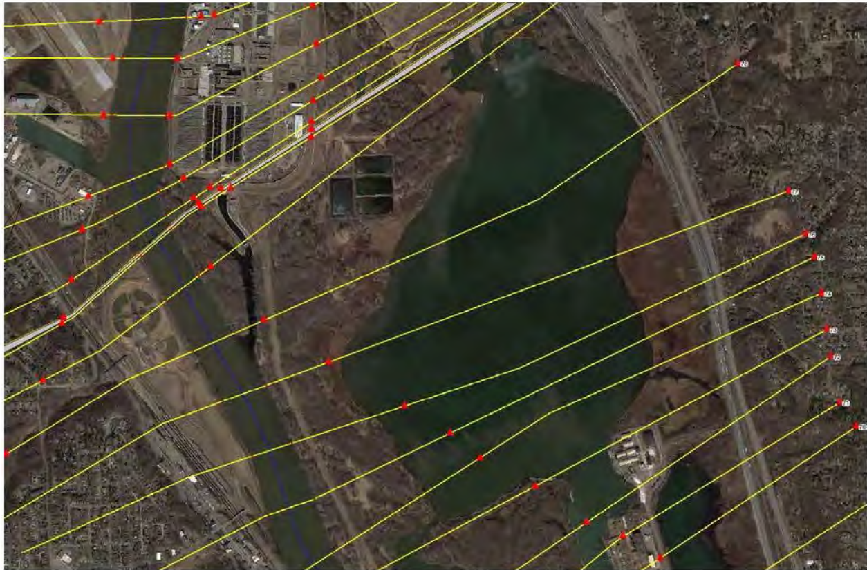
Figure 11 HEC-RAS Cross Sections (Ineffective Flow Boundary Shown in Red)
