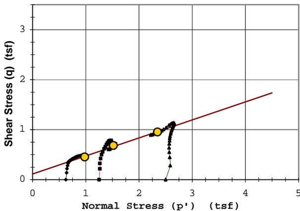
Rupture Envelope at Failure
