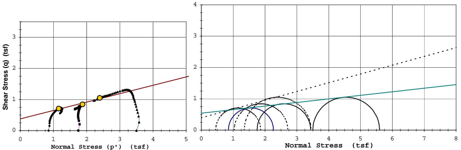
Rupture Envelope at Failure
