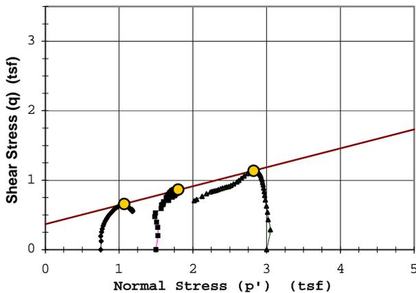
Rupture Envelope at Failure
