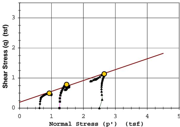
Rupture Envelope at Failure
