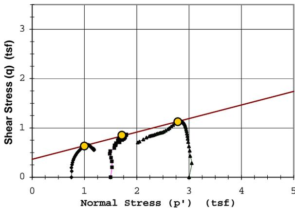
Rupture Envelope at Failure
