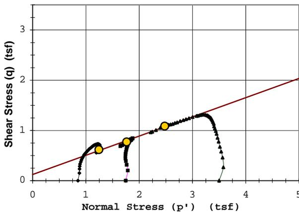
Rupture Envelope at Failure
