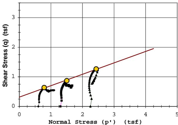
Rupture Envelope at Failure
