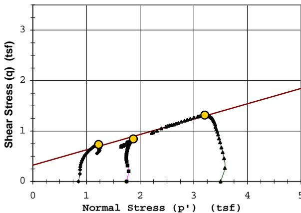
Rupture Envelope at Failure
