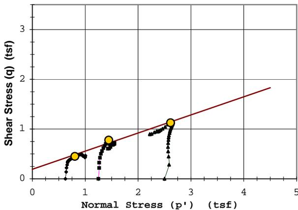
Rupture Envelope at Failure
