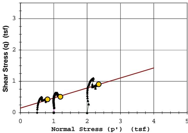
Rupture Envelope at Failure
