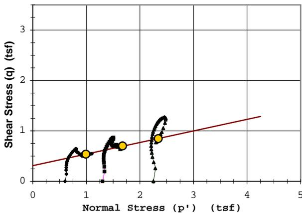
Rupture Envelope at Failure
