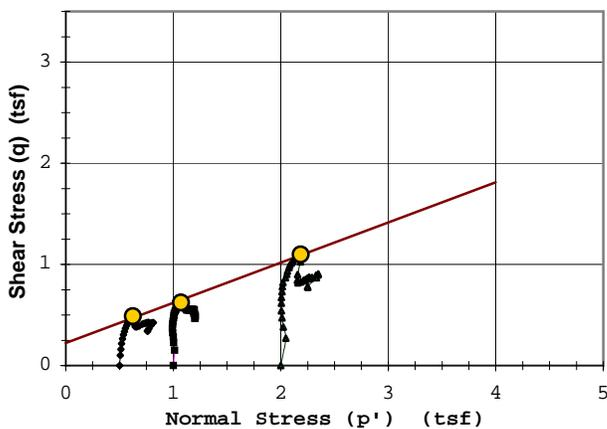
Rupture Envelope at Failure
