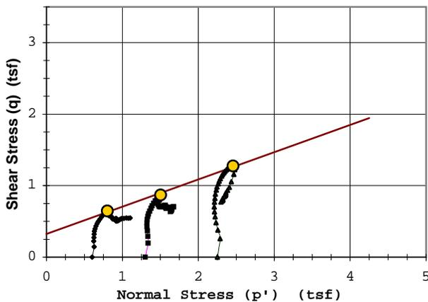
Rupture Envelope at Failure
