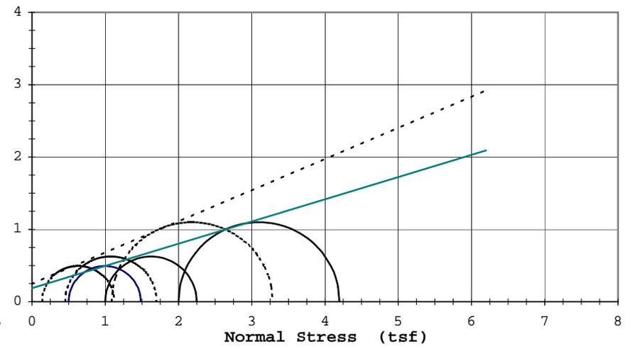
Rupture Envelope at Failure
