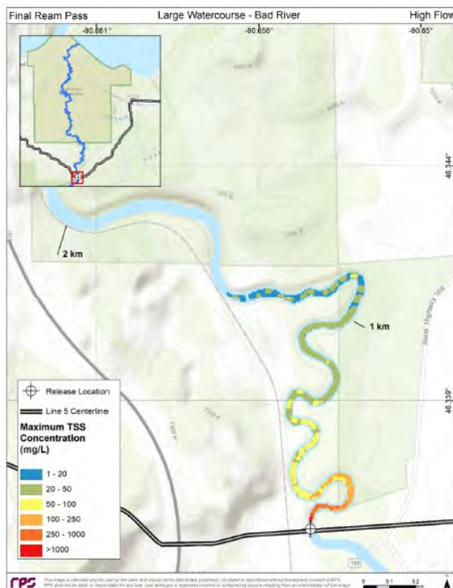
Figure 5-10. Maximum TSS concentrations above background predicted at any time in the simulation for the Final Ream scenario in high flow conditions. Downstream distance is provided on the map for reference (1 km = 0.62 miles; 2 km = 1.24 miles).
