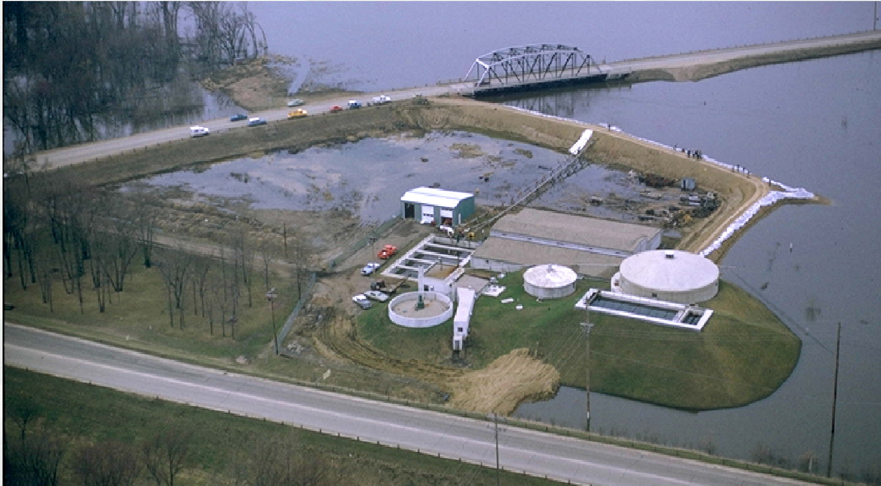
Aerial photo showing interior drainage blocked by levee
