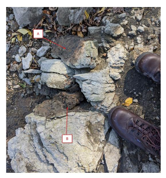
Figure 7 Rock at (A) dislodged with a few boot kicks from (B)
