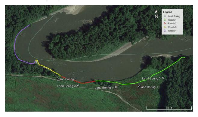
Figure 10 Proposed boring plan
